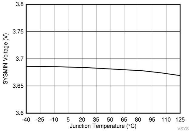
**Figure 7-7. SYSMIN Voltage vs Junction Temperature (V<sub>SY</sub> set at 3.5 V)**
