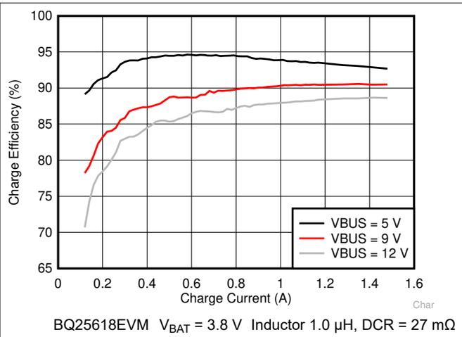
**Figure 7-2. Charge Efficiency**
