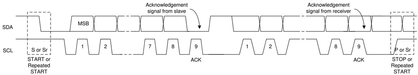
Figure 8-8. Data Transfer on the I<sup>2</sup>C Bus
