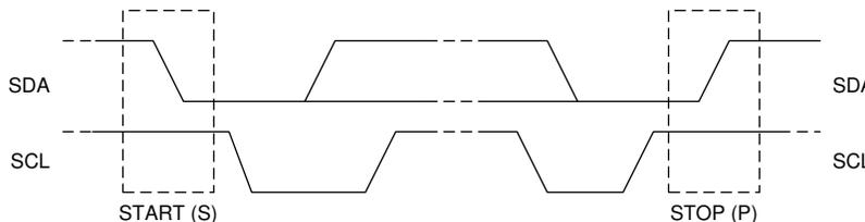
**Figure 8-7. TS START and STOP conditions**
