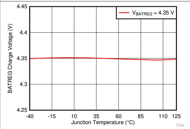
**Figure 7-4. Battery Charge Voltage vs Junction Temperature**
