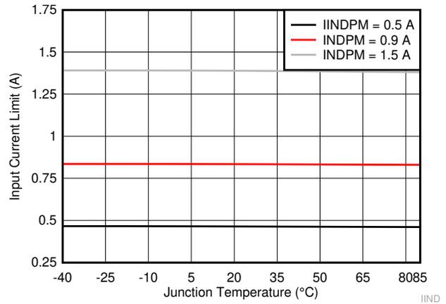
**Figure 7-8. Input Current Limit vs Junction Temperature**
