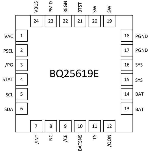
**Figure 6-2. BQ25619E RTW Package 24-Pin WQFN Top View**
