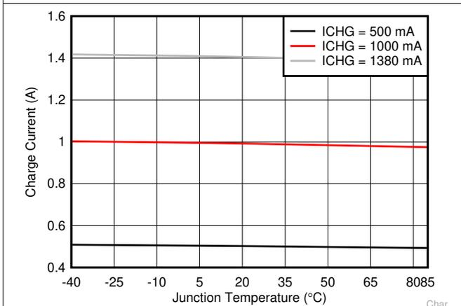
**Figure 7-5. Charge Current vs Junction Temperature**
