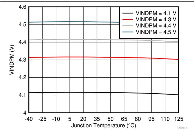
**Figure 7-6. VINDPM vs Junction Temperature**
