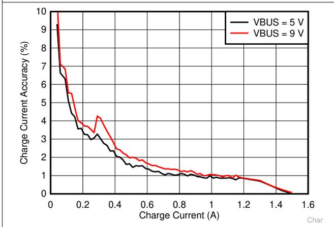
**Figure 7-3. Charge Current Accuracy**
