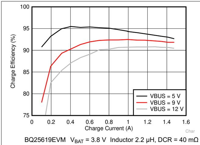
**Figure 7-1. Charge Efficiency**
