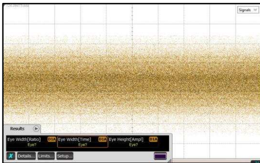
Figure 27. TL = 7-Meter 30-AWG 100 Ω Twin-Axial Cable, No Repeater, 10.3125 Gbps
