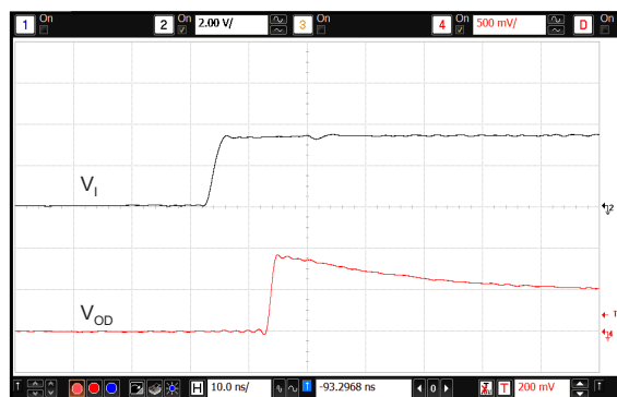
Figure 15. Distortion Correction Scheme Calibration Time (t CALIB )
