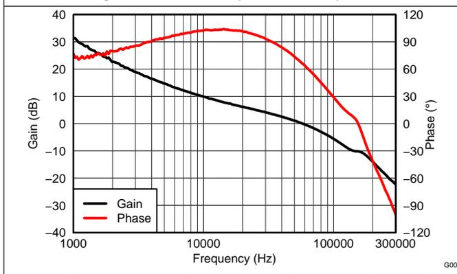
Figure 11. V<sub>OUT</sub> = 5 V, I<sub>OUT</sub> = 2 A, C<sub>OUT1</sub> = 44 μF ceramic, C<sub>OUT2</sub> = 56 μF electrolytic, f<sub>SW</sub> = 500 kHz
