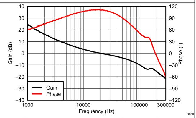
Figure 12. V<sub>OUT</sub> = 12 V, I<sub>OUT</sub> = 2 A, C<sub>OUT1</sub> = 44 μF ceramic, C<sub>OUT2</sub> = 56 μF electrolytic, f<sub>SW</sub> = 800 kHz
