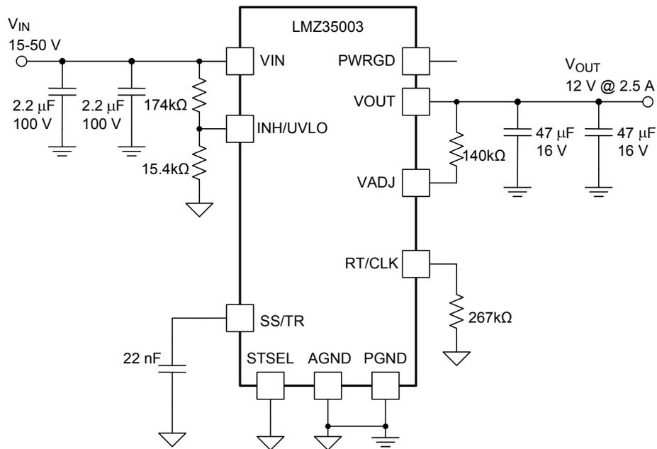
**Figure 29. Typical Schematic**
