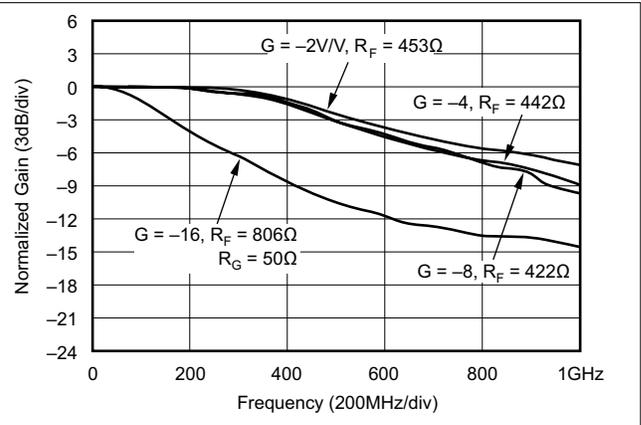
图 5-70. Inverting Small-Signal Frequency Response
