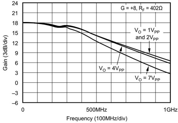
图 5-41. Noninverting Large-Signal Frequency Response
