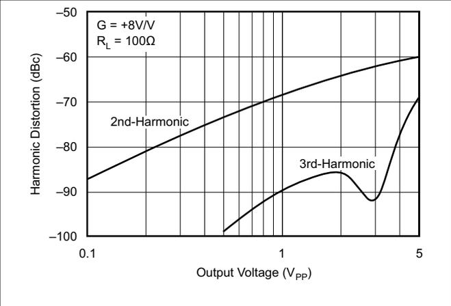
图 5-48. 10-MHz Harmonic Distortion vs Output Voltage
