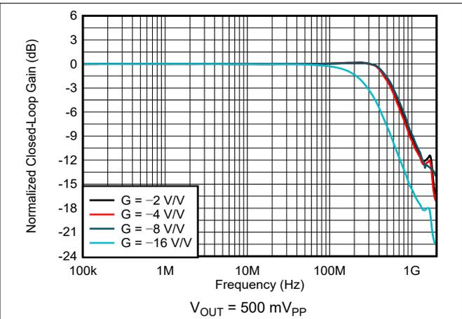
图 5-2. Inverting Small-Signal Frequency Response
