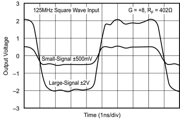
图 5-44. Inverting Large- and Small-Signal Frequency Responses
