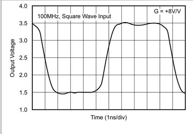
图 5-71. Noninverting Pulse Response
