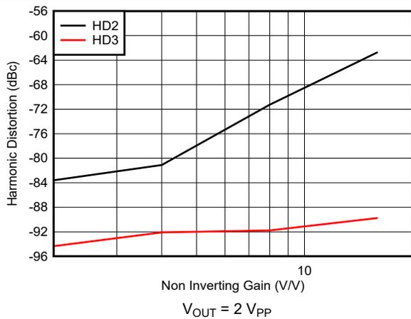
图 5-11. 10-MHz Harmonic Distortion vs Noninverting Gain
