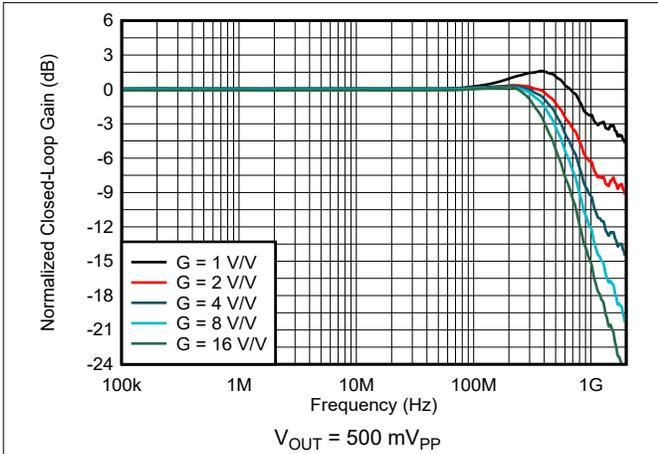
图 5-29. Noninverting Small-Signal Frequency Response
