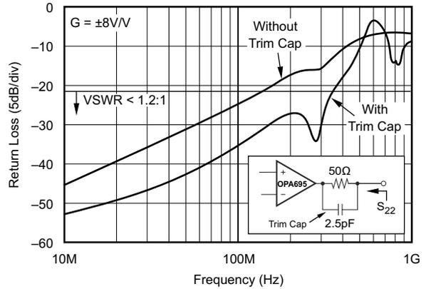
图 5-54. Output Return Loss vs Frequency ( $S_{22}$ )
