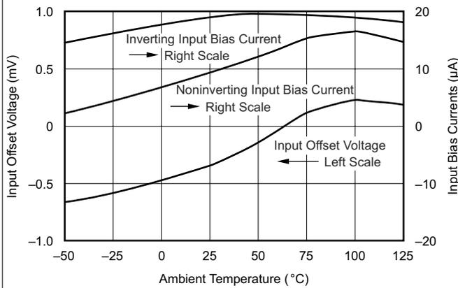
图 5-65. Typical DC Drift Over Temperature
