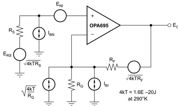
图 7-4. Operational Amplifier Noise Figure Analysis Model
