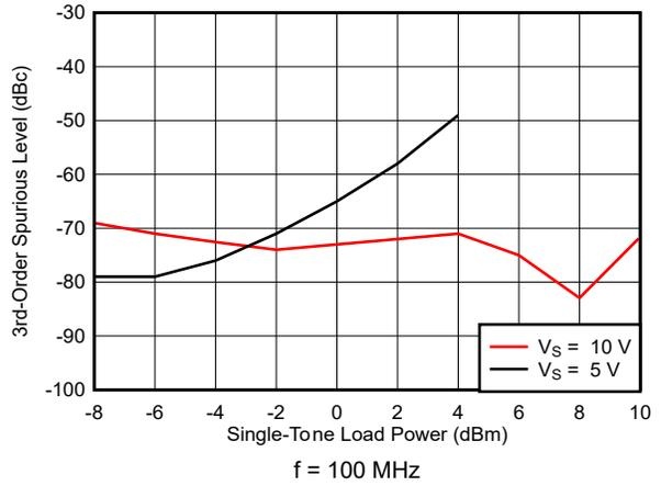
图 5-14. Two-Tone 3rd-Order Intermodulation Distortion vs Frequency
