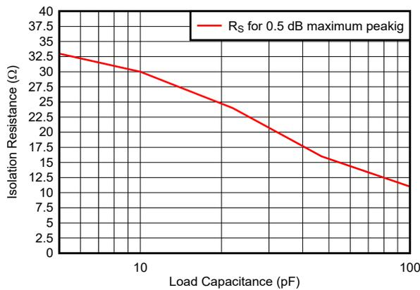
图 5-17.  $R_S$  vs Capacitive Load
