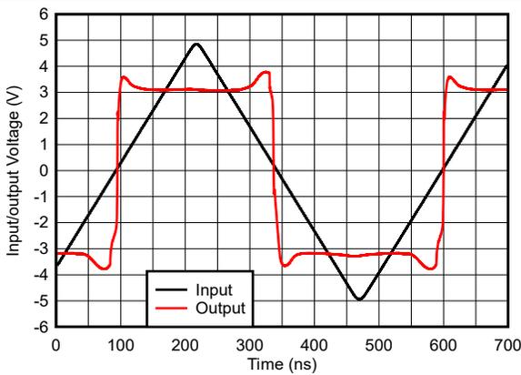
图 5-23. Noninverting Overdrive Recovery
