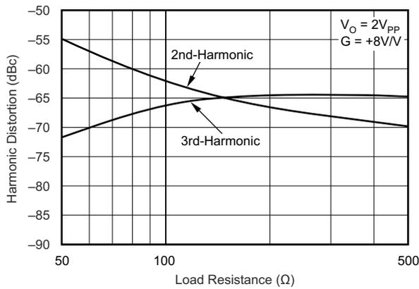
图 5-77. 10-MHz Harmonic Distortion vs Load Resistance
