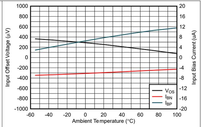
图 5-26. Typical DC Drift Over Temperature
