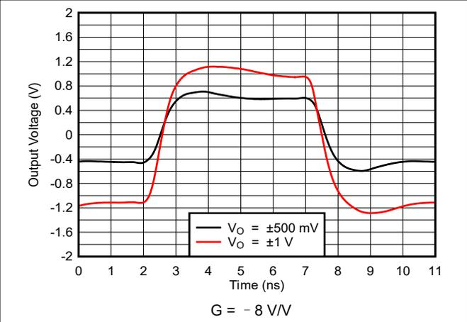
图 5-32. Inverting Pulse Response
