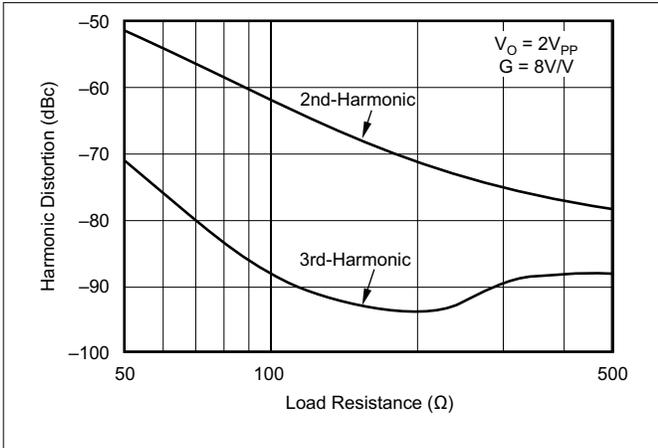
图 5-45. 10-MHz Harmonic Distortion vs Load Resistance
