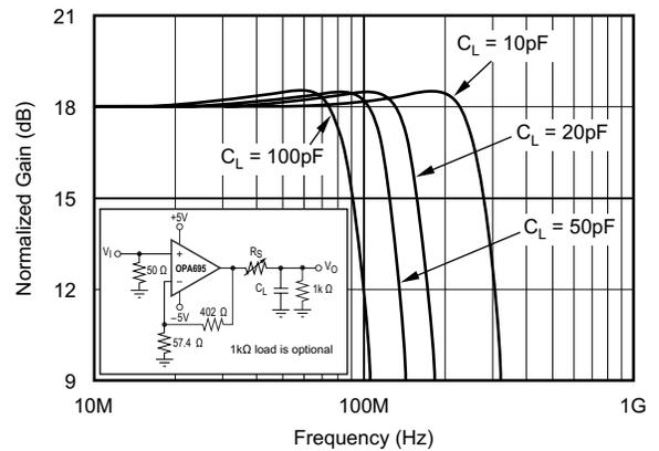
图 5-56. Small-Signal Frequency Response vs Capacitive Load
