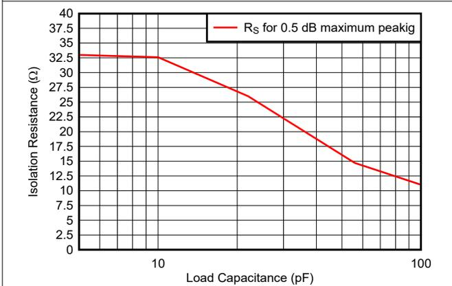
图 5-33.  $R_S$  vs Capacitive Load
