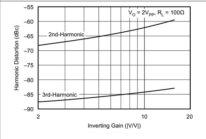
图 5-50. 10-MHz Harmonic Distortion vs Inverting Gain
