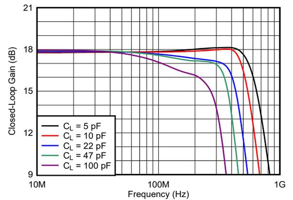
图 5-18. Small-Signal Frequency Response vs Capacitive Load
