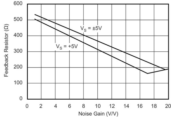
**图 7-2. Recommended Feedback Resistor vs Noise Gain**
