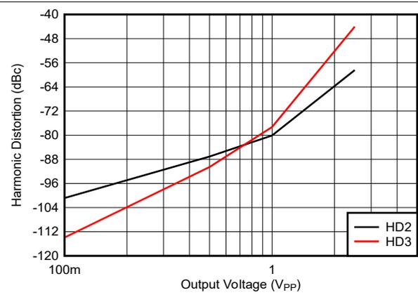
图 5-36. 10-MHz Harmonic Distortion vs Output Voltage
