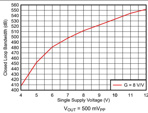
图 5-38. Small-Signal BW vs Single-Supply Voltage
