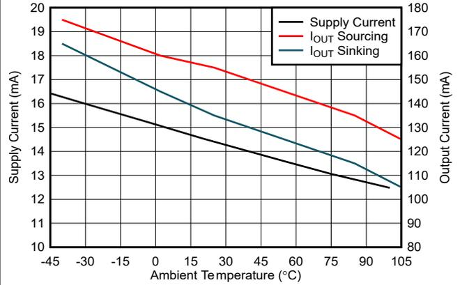
图 5-22. Supply and Output Current vs Temperature
