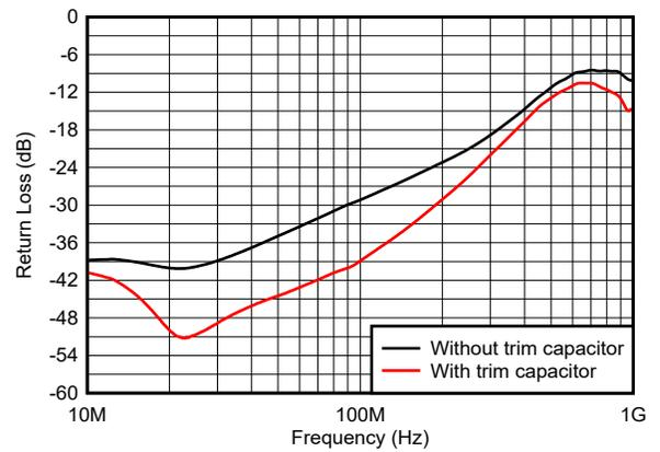
图 5-16. Output Return Loss vs Frequency ( $S_{22}$ )
