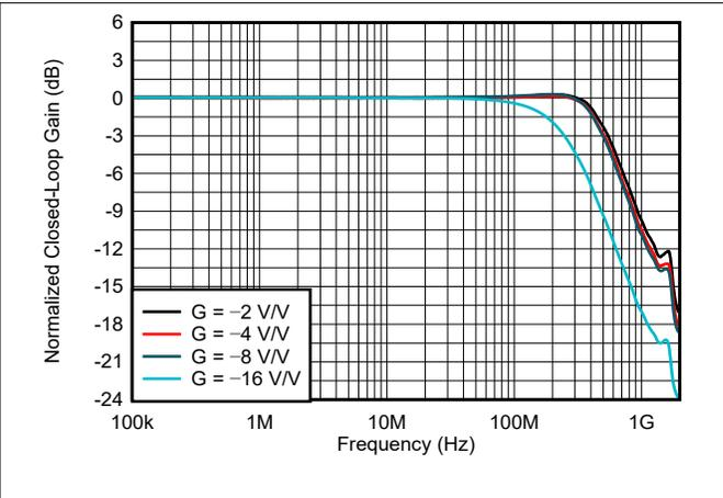
图 5-30. Inverting Small-Signal Frequency Response
