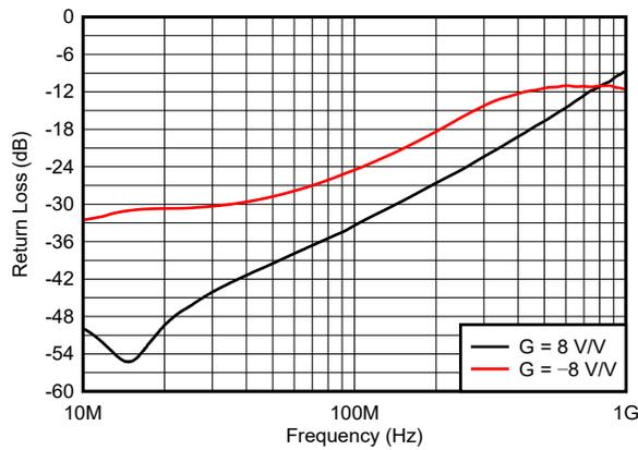
图 5-15. Input Return Loss vs Frequency ( $S_{11}$ )
