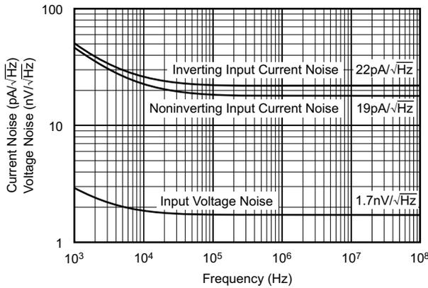
图 5-51. Input Voltage and Current Noise Density
