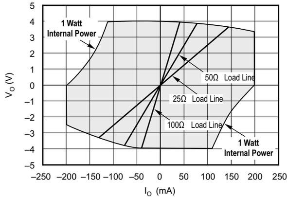
图 5-59. Output Voltage and Current Limitations
