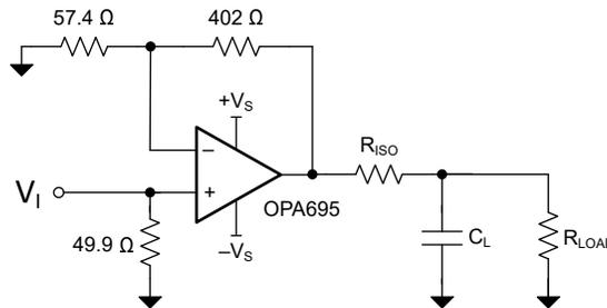
图 7-3. Driving a Large Capacitive Load Using an Output Series Isolation Resistor
