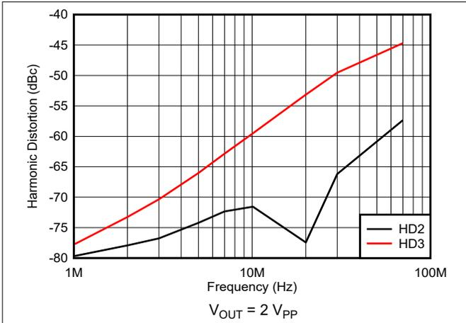
图 5-35. Harmonic Distortion vs Frequency
