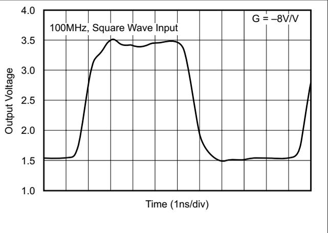
图 5-72. Inverting Pulse Response
