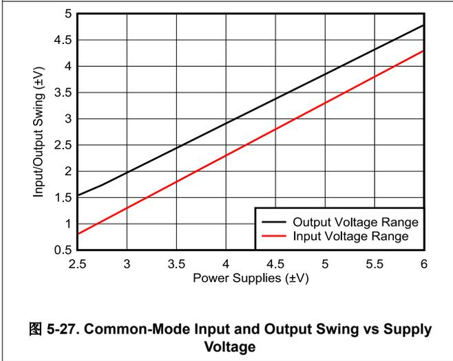
图 5-27. Common-Mode Input and Output Swing vs Supply Voltage
