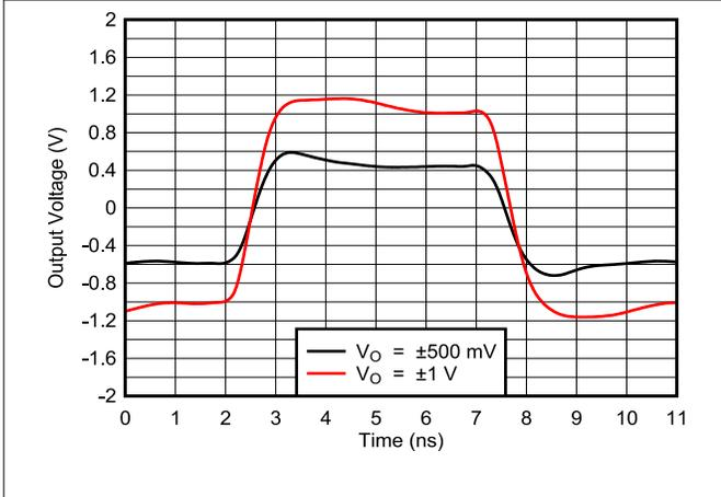
图 5-31. Noninverting Pulse Response
