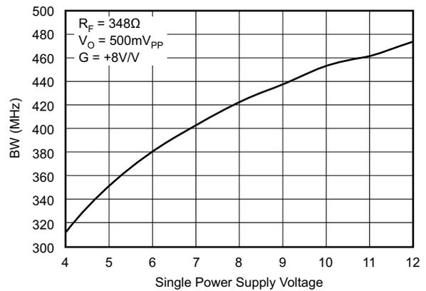
图 5-68. Small-Signal BW vs Single-Supply Voltage
