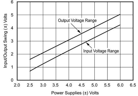
图 5-66. Common-Mode Input and Output Swing vs Supply Voltage
