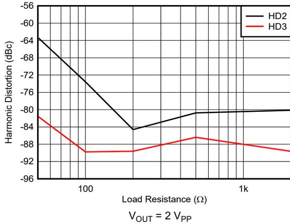
图 5-7. 10-MHz Harmonic Distortion vs Load Resistance
