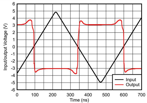
图 5-24. Inverting Overdrive Recovery
