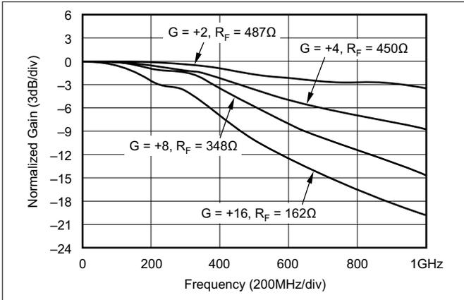
图 5-69. Noninverting Small-Signal Frequency Response
