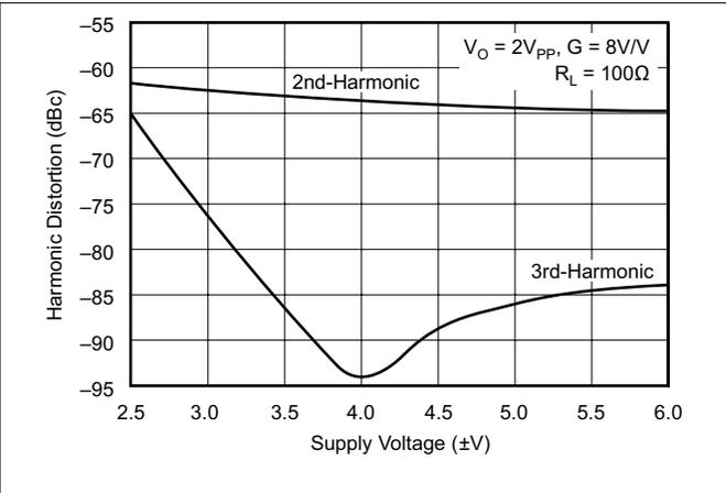
图 5-46. 10-MHz Harmonic Distortion vs Supply Voltage
