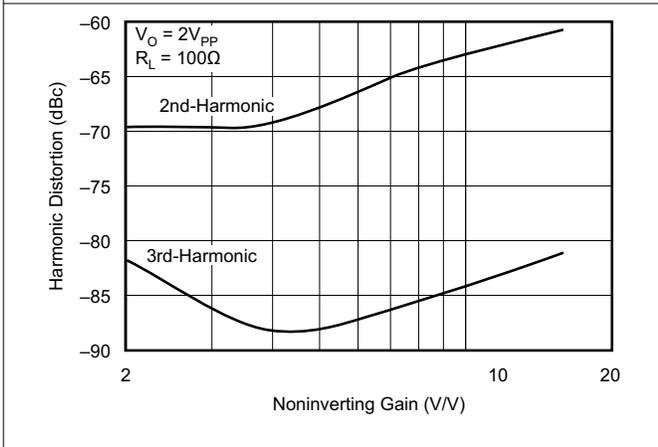
图 5-49. 10-MHz Harmonic Distortion vs Noninverting Gain
