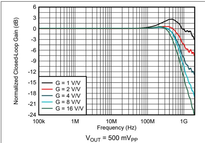
图 5-1. Noninverting Small-Signal Frequency Response
