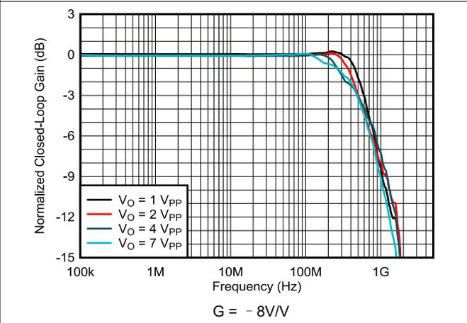
图 5-4. Inverting Large-Signal Frequency Response
