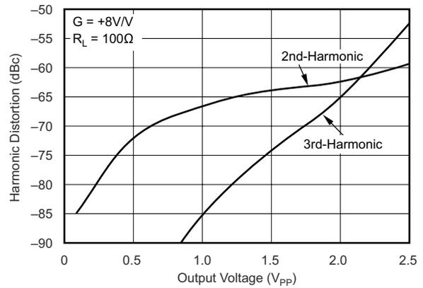
图 5-76. 10-MHz Harmonic Distortion vs Output Voltage
