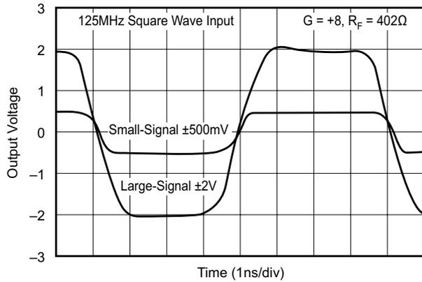
图 5-43. Noninverting Large- and Small-Signal Frequency Responses
