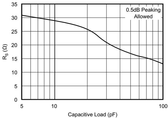
图 5-55.  $R_S$  vs Capacitive Load
