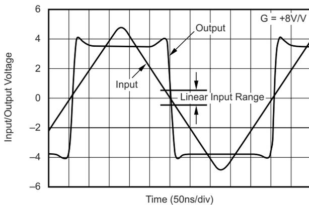
图 5-61. Noninverting Overdrive Recovery
