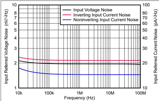
图 5-13. Input Voltage and Current Noise Density
