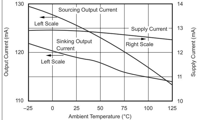
图 5-60. Supply and Output Current vs Temperature
