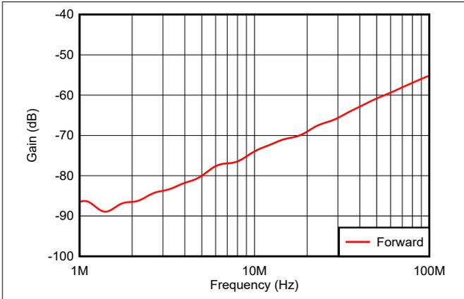
图 5-25. Disabled Feedthrough vs Frequency
