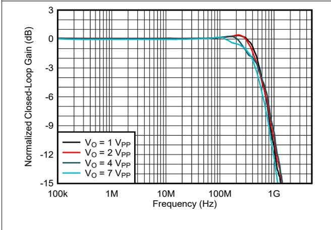
图 5-3. Noninverting Large-Signal Frequency Response
