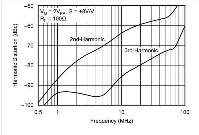
图 5-47. Harmonic Distortion vs Frequency
