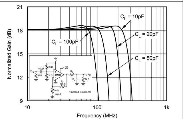
图 5-74. Small-Signal Frequency Response vs Capacitive Load
