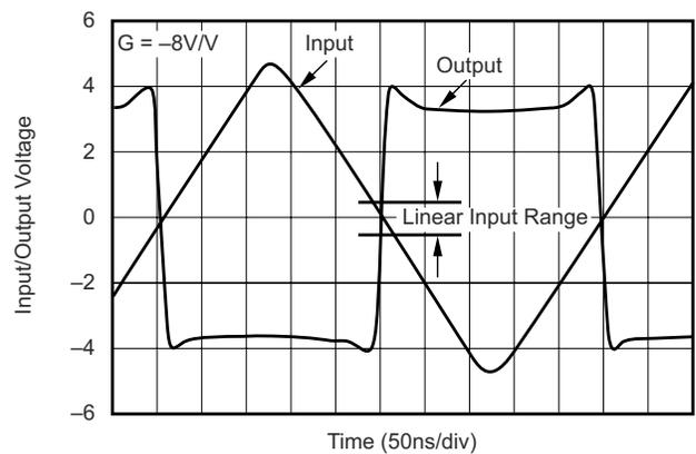
图 5-62. Inverting Overdrive Recovery
