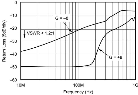
图 5-53. Input Return Loss vs Frequency ( $S_{11}$ )
