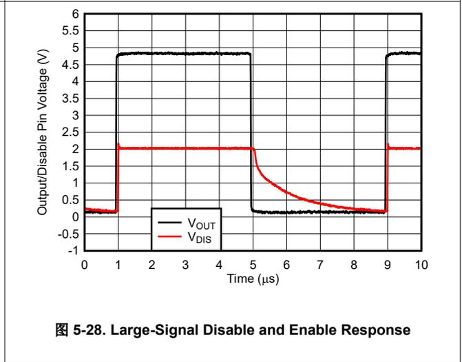
图 5-28. Large-Signal Disable and Enable Response
