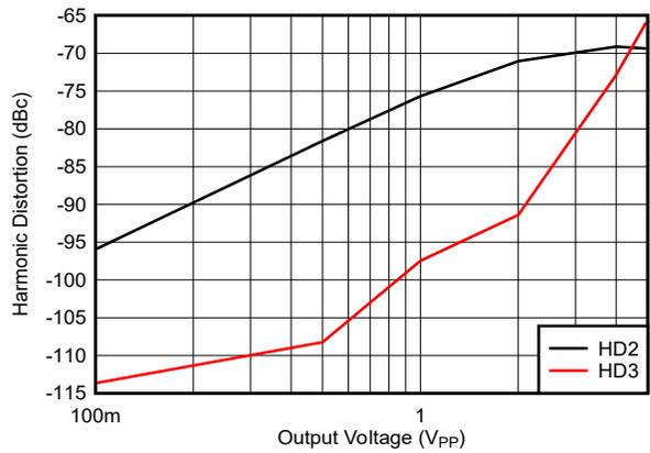
图 5-10. 10-MHz Harmonic Distortion vs Output Voltage
