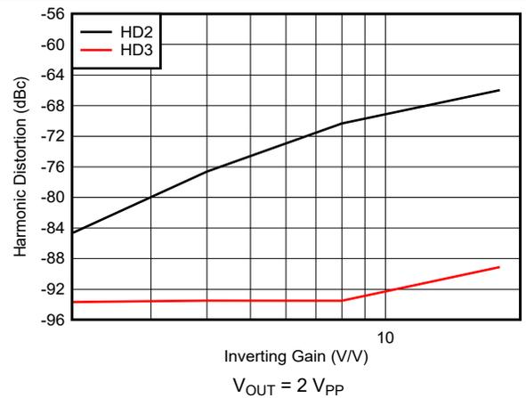
图 5-12. 10-MHz Harmonic Distortion vs Inverting Gain
