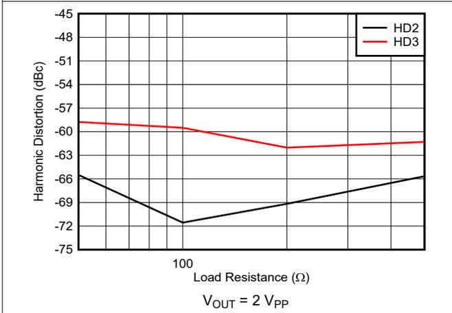
图 5-37. 10-MHz Harmonic Distortion vs Load Resistance
