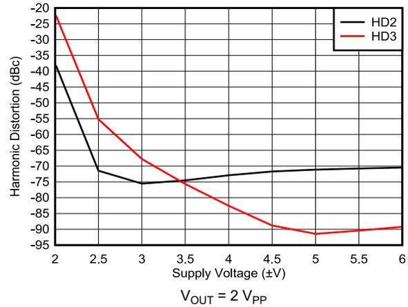
图 5-8. 10-MHz Harmonic Distortion vs Supply Voltage
