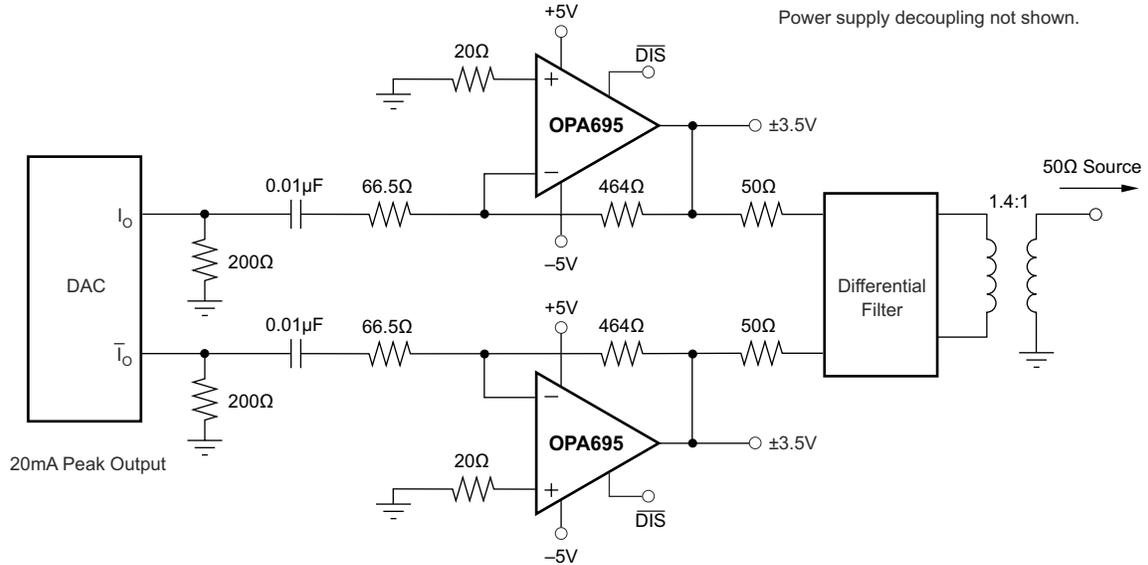
图 7-7. High Power, Wideband AC-Coupled Arbitrary Waveform Driver
