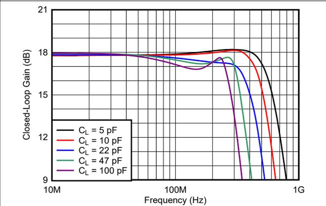
图 5-34. Small-Signal Frequency Response vs Capacitive Load
