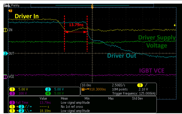
图 8-3. UCC27624 Used to Drive IGBT in the Boost Converter
