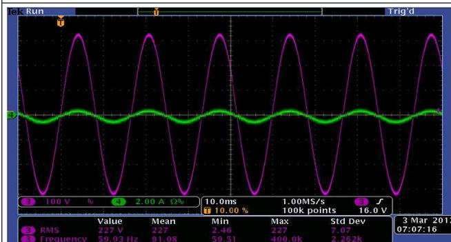
Ch3-Vin, Ch4-Iin, Vrms = 230V, Vbus = 390V, Pout = 80W
