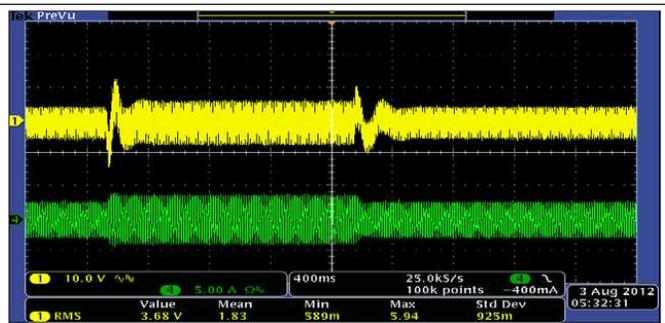
Ch1-Vbus, Ch4-Iin, Vrms = 220V, Vbus = 390V, Load Step 370W ~ 530W
