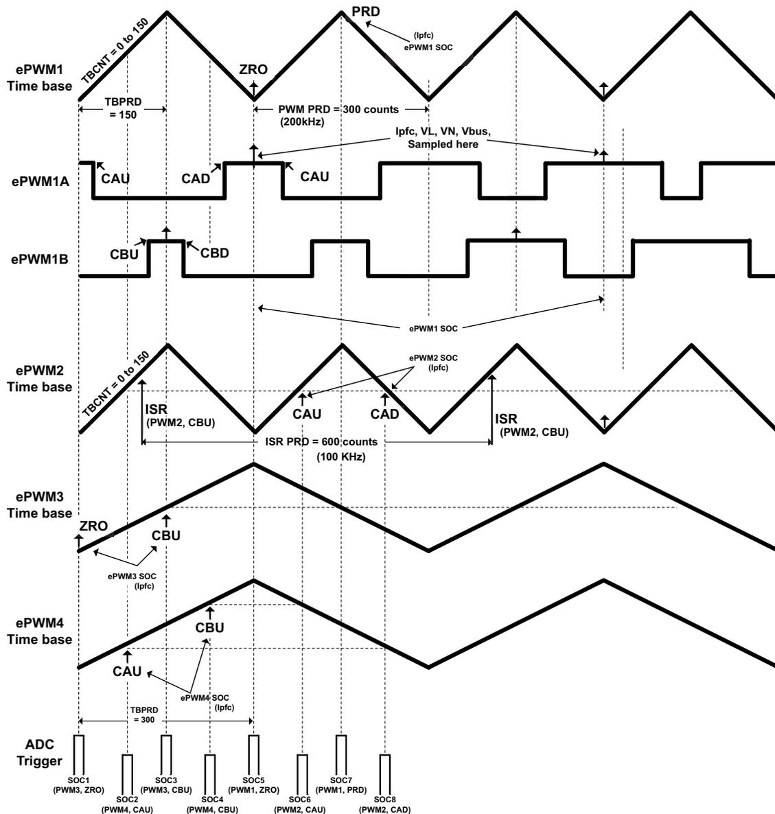
图 8. PWM generation and ADC Sampling
