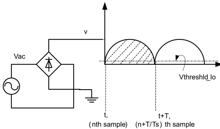
图 13. RMS Input Voltage and Current Calculation Scheme
