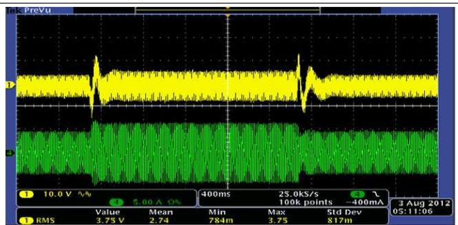
Ch1-Vbus, Ch4-Iin, Vrms = 120V, Vbus = 390V, Load Step 360W ~ 520W
