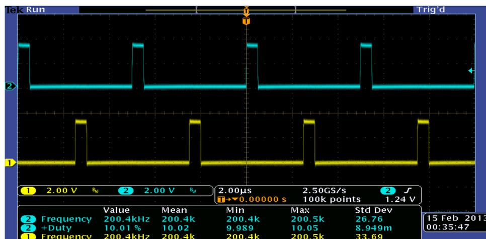
8. Try different duty cycle values and observe the corresponding ADC results. Increase duty cycle value in small steps. Always observe the output voltage carefully, this should not be allowed to exceed the capabilities of the board. Different waveforms, like the PWM gate drive signals, input voltage and current and output voltage may also be probed and verified using an oscilloscope. Appropriate safety measures must be taken while probing these high voltage signals.
