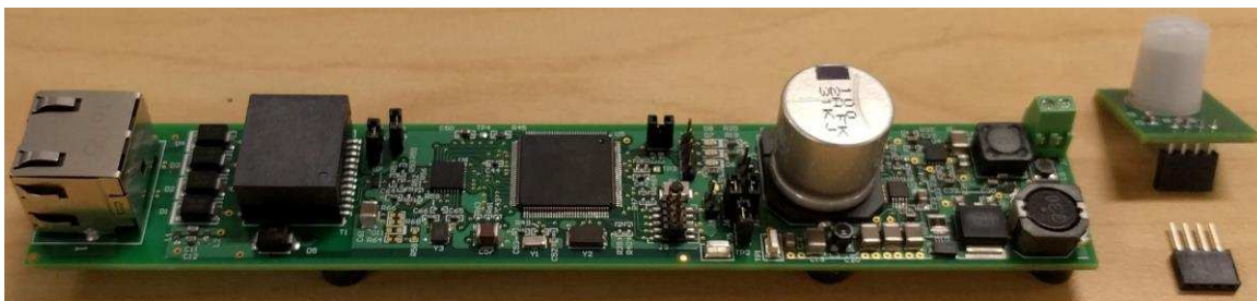
图 9. TIDA-01463 PCB With IR Sensor
