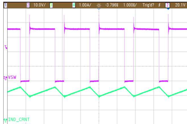
图 16. Buck Stage Switching Waveform
