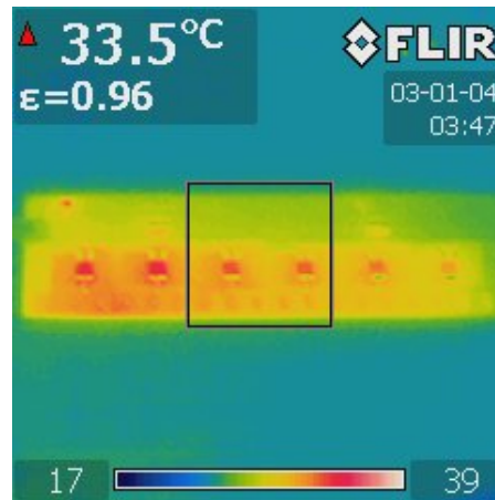
图 11. Thermal Image of Tail-Light Function at 25°C, 12-V Input Voltage
