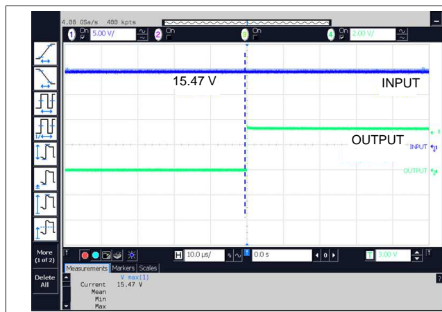
图 9. High-Level Threshold Voltage of TIDA-060014
