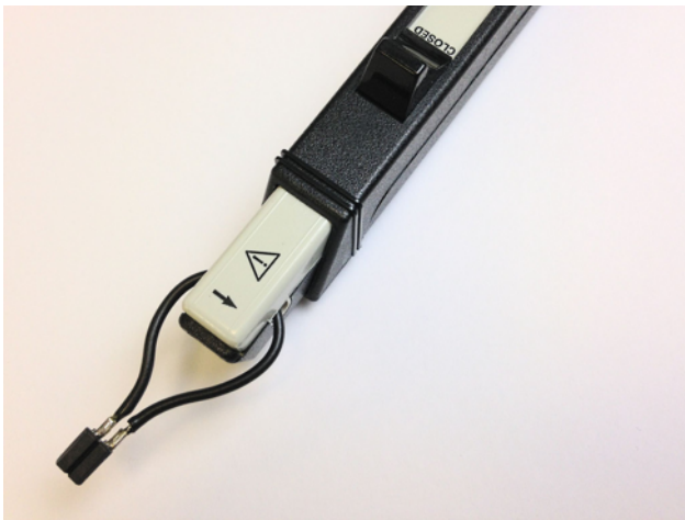
图 18. Current Probe with Self-made Adapter Wire for Primary Winding Current Measurement
