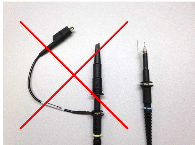
图 19. Probe With Long Ground Lead and Alligator Clip vs Probe With Ground Spring
