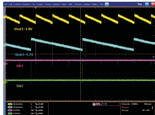
Figure 12. Buck 1 and Buck 2 in PSM Mode
