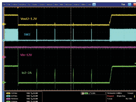
Figure 13. Buck 2 Hard Short and Recover
