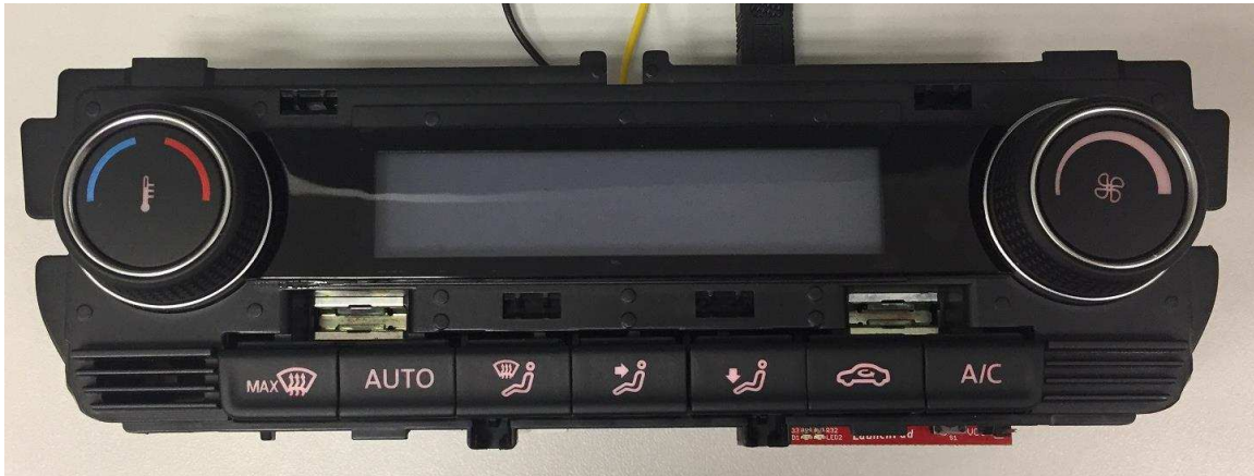
図 18. LED Dimming With 4% Duty Cycle
