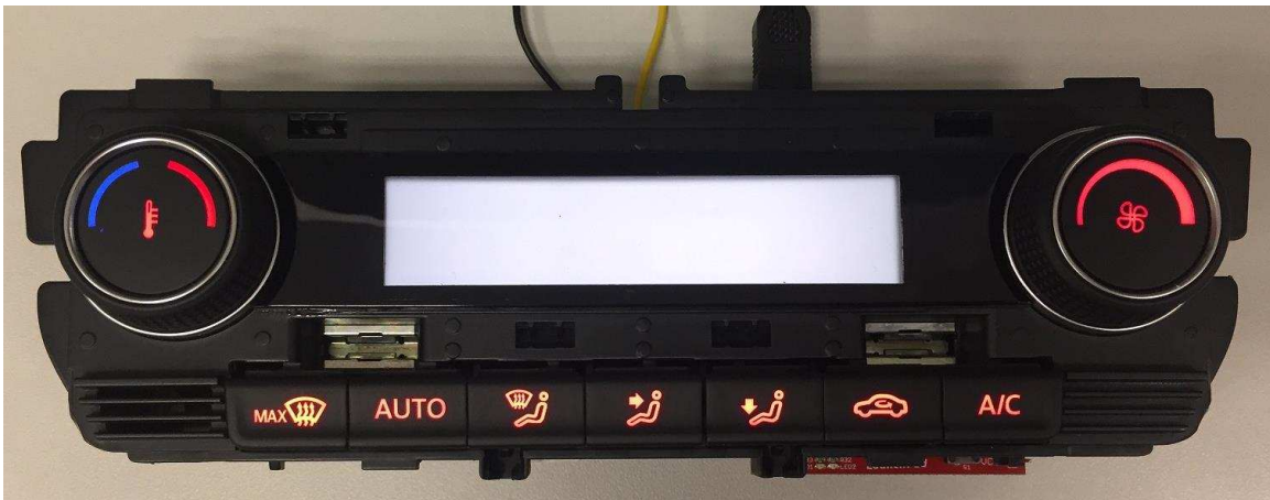
図 21. LED Dimming With 80% Duty Cycle
