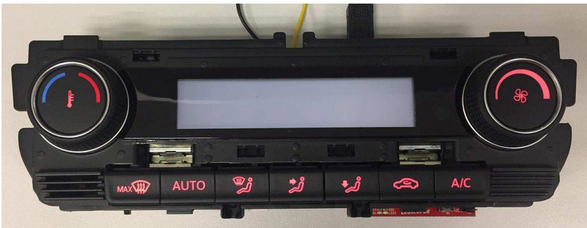
図 19. LED Dimming With 20% Duty Cycle
