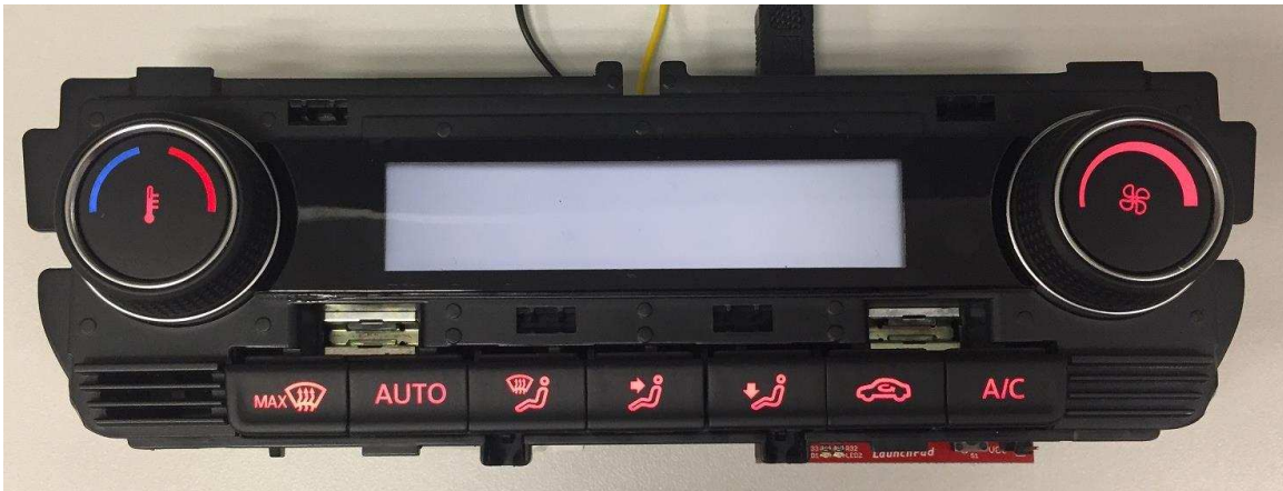
図 20. LED Dimming With 45% Duty Cycle
