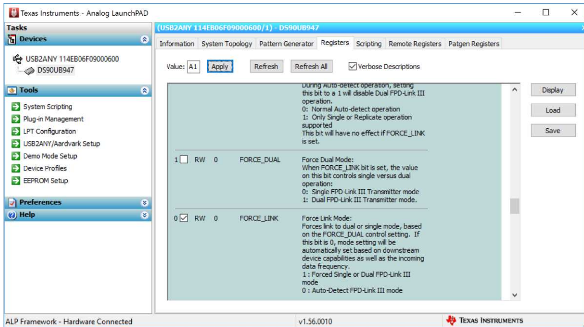
Figure 16. DS90UB947-Q1 Register 0x5B.1:0=01
