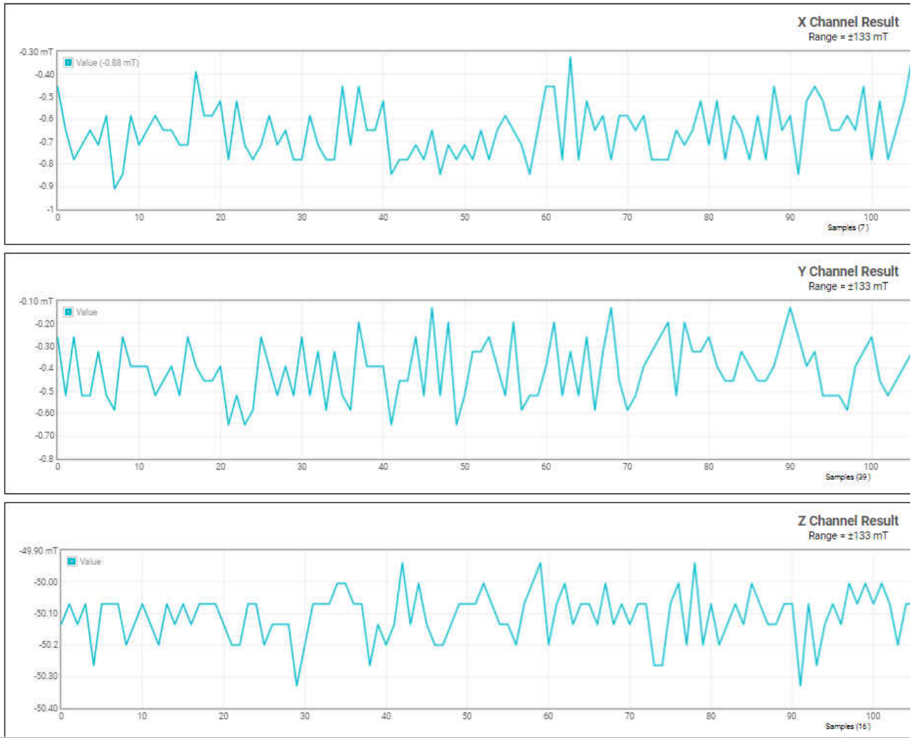
Figure 4-2. Magnetic Flux Density Results when Screw is Fully Fastened into Base
