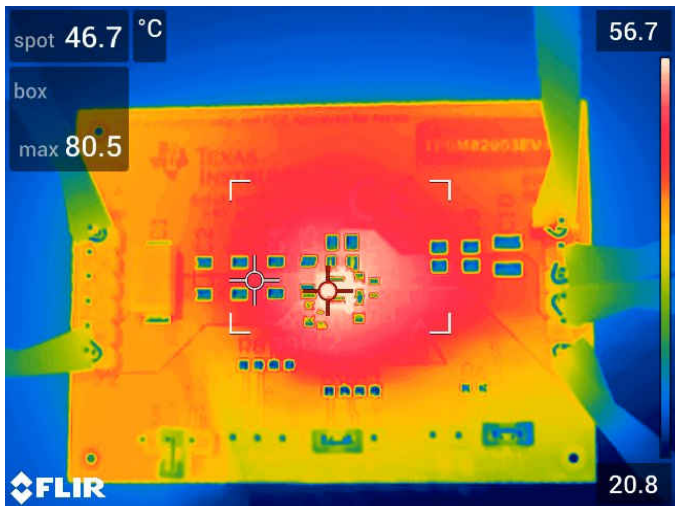
Figure 4-1. Thermal Performance ( V_{IN} = 12\text{ V} , V_{OUT} = 1.2\text{ V} , I_{OUT} = 3000\text{ mA} , JP3 Open)
