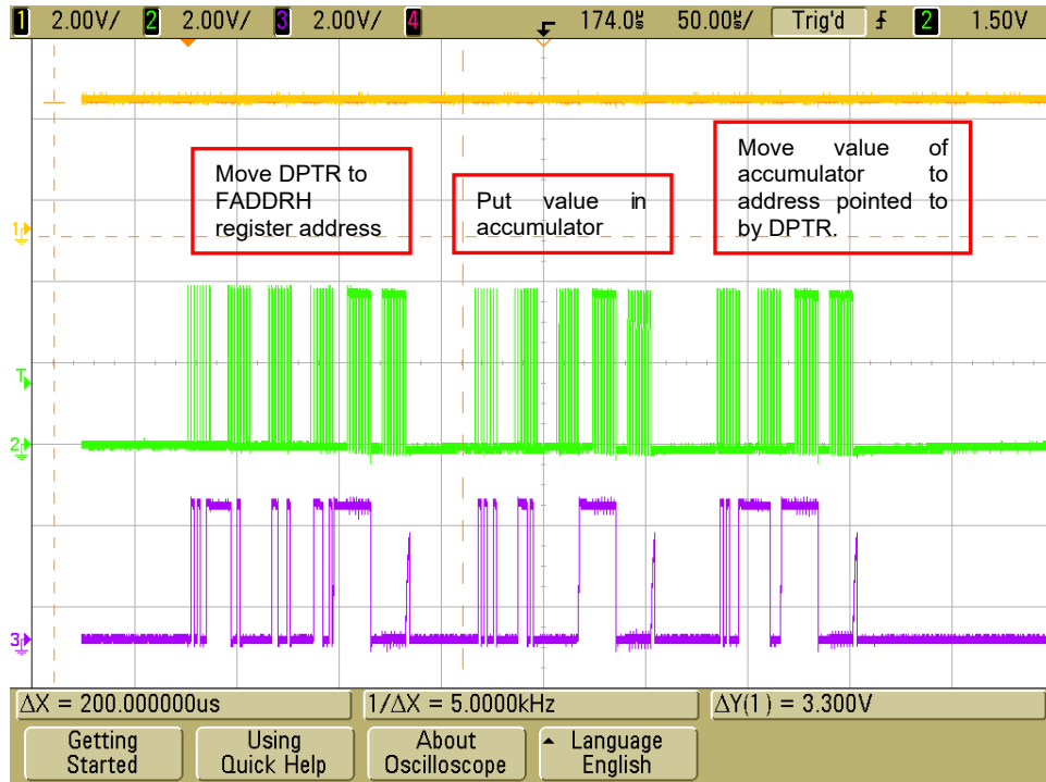
Figure 8 – Writing 8 MSb [17:10] of 18-bit flash start address to FADDRH
