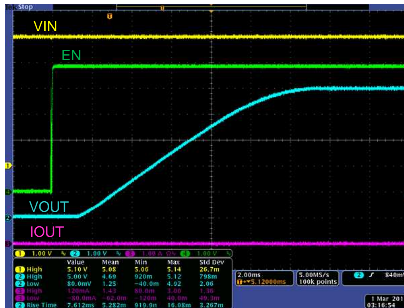
Figure 6. Soft Start Behavior With No Load
