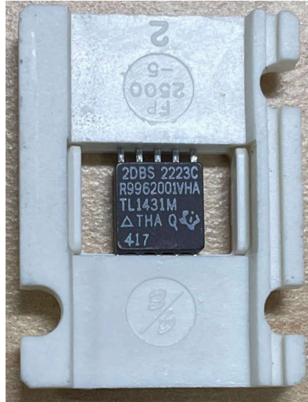
Figure 2-1. TL1431-SP Device (Front)
