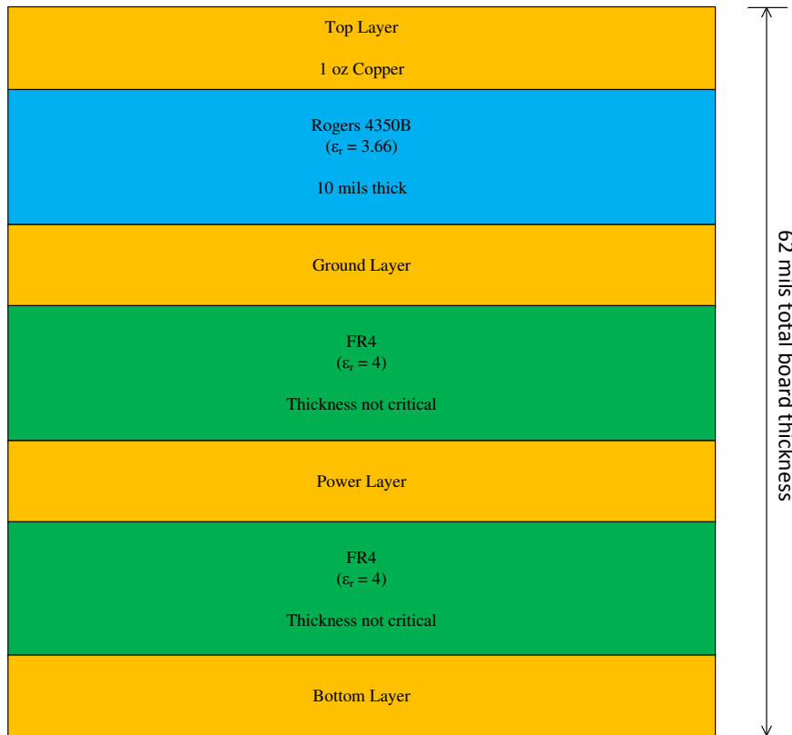
Figure 8-1. Board Layer Stack-Up
