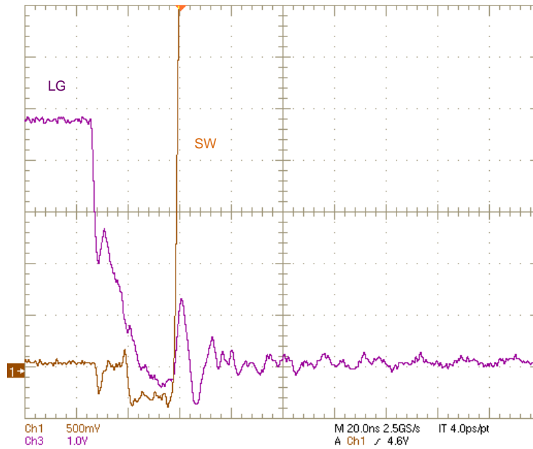
Figure 22. Deadtime Prior To High-side MOSFET Turn-on; V_{IN} = 12\text{ V} , V_{OUT} = 1.2\text{ V} , 120-m \Omega Load
