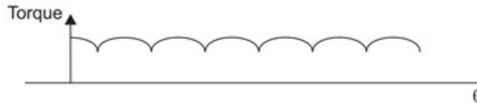
Figure 3. Torque Ripple When a PMSM Is Driven as a BLDC Motor Using Six-step Commutation
