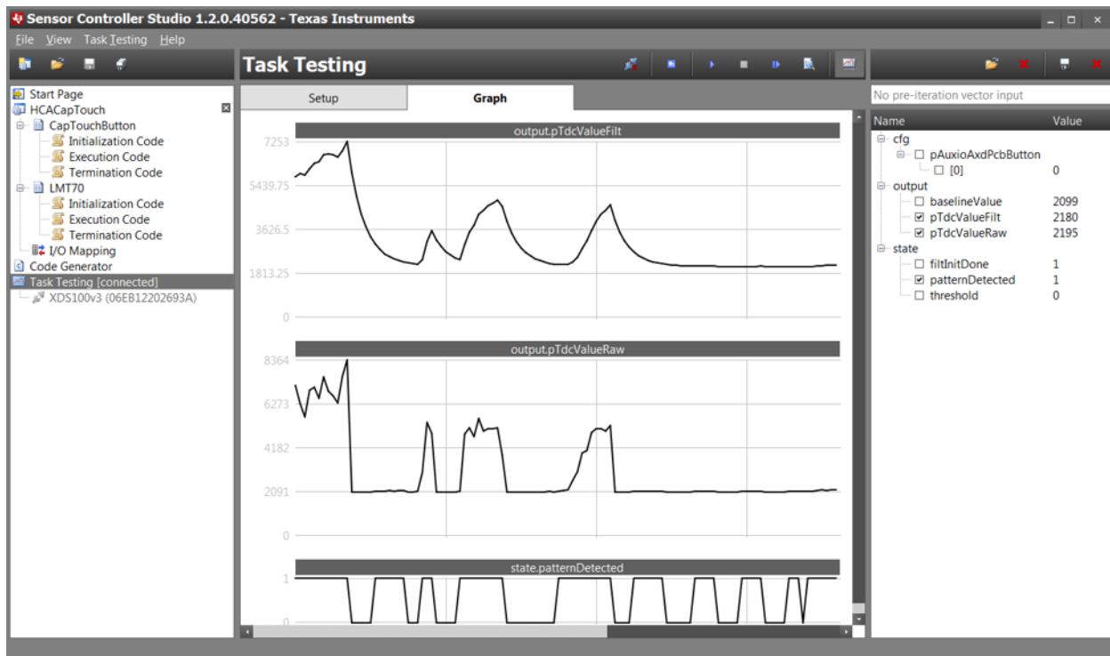
Figure 13. Task Testing Under SCS: Touch Events are the Peaks in the Two Upper Graphs
