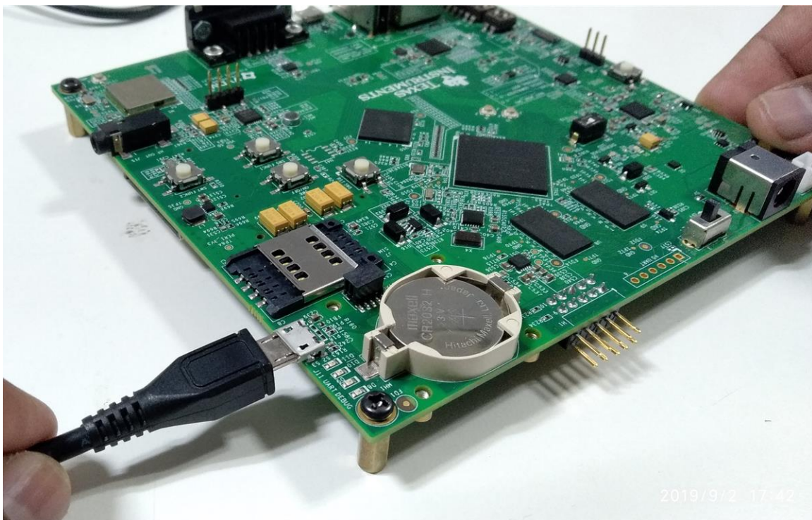
Figure 27. Inserting micro-B Cable Into J11
